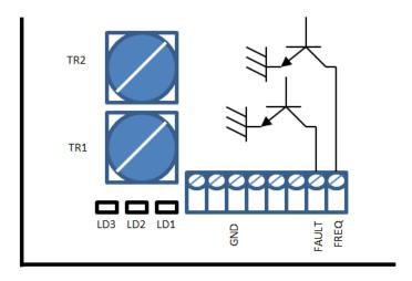
**Note:** The FAULT output is normally closed. It opens when an alarm happens. In the case of the pull up resistor, the alarm output is a voltage (+12 Vdc signal).
