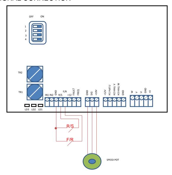
Connect the potentiometer as shown in diagram. Be careful: the cursor (variable pin) must be connected to SIG. in case of analog power supply 0/+10 V, the reference goes to GND and the signal to SIG.
